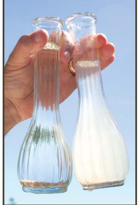
**At left is natural sand from a beach north of Fort Pierce Inlet; at right is offshore borrow material that was pumped onto Martin County beaches. Given a shake, the natural sand settled out in seconds, while the borrow material fouled the water indefinitely.**
